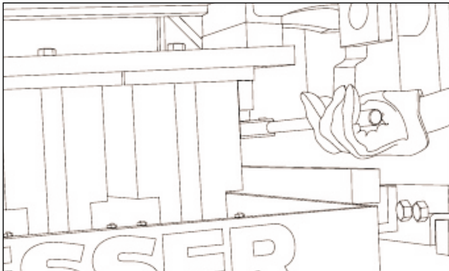
Figure 5.3 REMOVING BOLTS FROM BOLT STRIPPER HEAD PLATE.
