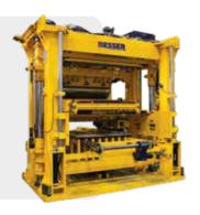
The original Servopac®, the Classic was designed for versatility of production. Quick mold and height changes, along with independent control of frequency and amplitude in the vibration system allows the Classic to produce a wide variety of products through minimal human touches. This flexibility makes it easy to integrate short runs into the production schedule. Production versatility makes the Classic the perfect machine for producers consolidating plants.
