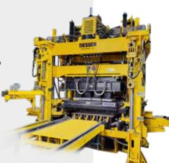
The Premier is a traditional big board machine, with Besser ingenuity. It is the first and only big board machine engineered and manufactured in the United States. Standard Servo table (impact) vibration provides the operator with independent frequency and amplitude control.
