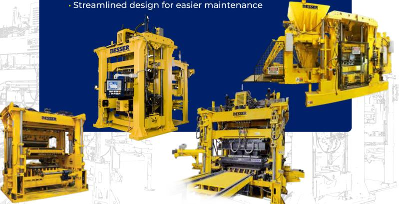
Introduced in 2018, the Select boasts select features from the Classic. Adapting the renowned Advanced Servo Vibration (ASV) from cam machines, the Select has two Servo motors for vibration which allow control of frequency.
