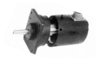
The Digisolver is a Rotary Sensor which provides the Programmable Logic Controller (PLC) with a "0" to "359" degree value. The unit operates on 24 VDC plus or minus 1.0 VDC and is connected with one of the following cable lengths (part number): 50 ft (113815); 60 ft (114014); 75 ft (114015): 100 ft (115114) or 150 ft (114182), between the Digisolver and input module 1:3. The word value may be monitored by using the ROTARY SENSOR screen.
