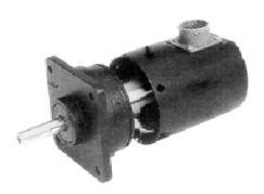
The DuraCoder is a Rotary Sensor which provides the Programmable Logic Controller (PLC) with a "0" to "359" degree value. The unit operates on 24 VDC and is connected with one of the following cable lengths (part number): 5 ft with male connector on one end and female connector on the other end (116146), 50 ft (113815); 60 ft (114014); 75 ft (114015): 100 ft (115114) or 150 ft (114182), between the DuraCoder and input module I:3. The word value may be monitored by using the ROTARY SENSOR screen.
