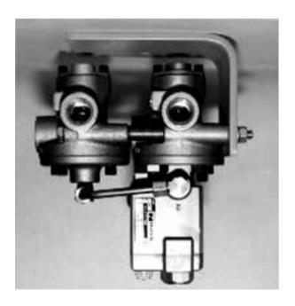
Besser has parts available to update your air valves to this NEW VALVE which allows operators to independently adjust the air pressure on the Clutch/Brake of the Bescodyne Drives. Simply replace the single air flow valve No. 107616 Ross Valve - 4 Way Directional Control, with the NEW DOUBLE AIR FLOW VALVE No. 103916.
