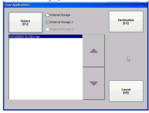
Then, highlight the mer file to be copied from the "External Storage 1". (If the mer file was not copied onto the SD Card into the proper directory, it will not show up for selection. As an example assuming the application file is 517281.mer is already copied to the SD Card, when viewing the card on a regular computer with windows explorer, you would see (assuming the SD card is mapped to E drive):
