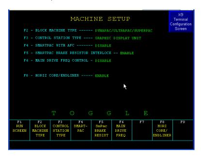
4. Touch "K9 Terminal Configuration Screen" to shutdown the project and launch FactoryTalk View ME Station, the Configuration mode of the terminal.
