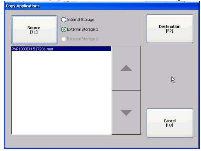
Then, highlight the mer file to be copied from the "External Storage 1". (If the mer file was not copied onto the SD Card into the proper directory, it will not show up for selection. As an example assuming the application file is 517281.mer is already copied to the SD Card, when viewing the card on a regular computer with windows explorer, you would see (assuming the SD card is mapped to E drive):
